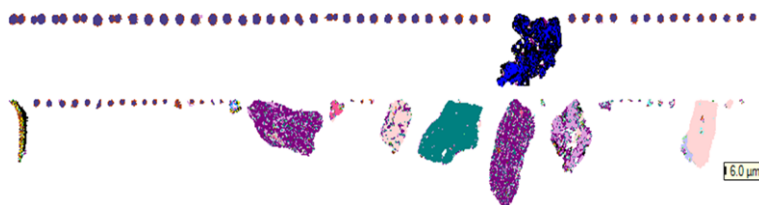
Fig. 7. QEMSCAN ® particle images for a spherical Ba–Sb phase present on the uppers of footwear item (b). The source of these particles is unknown.
