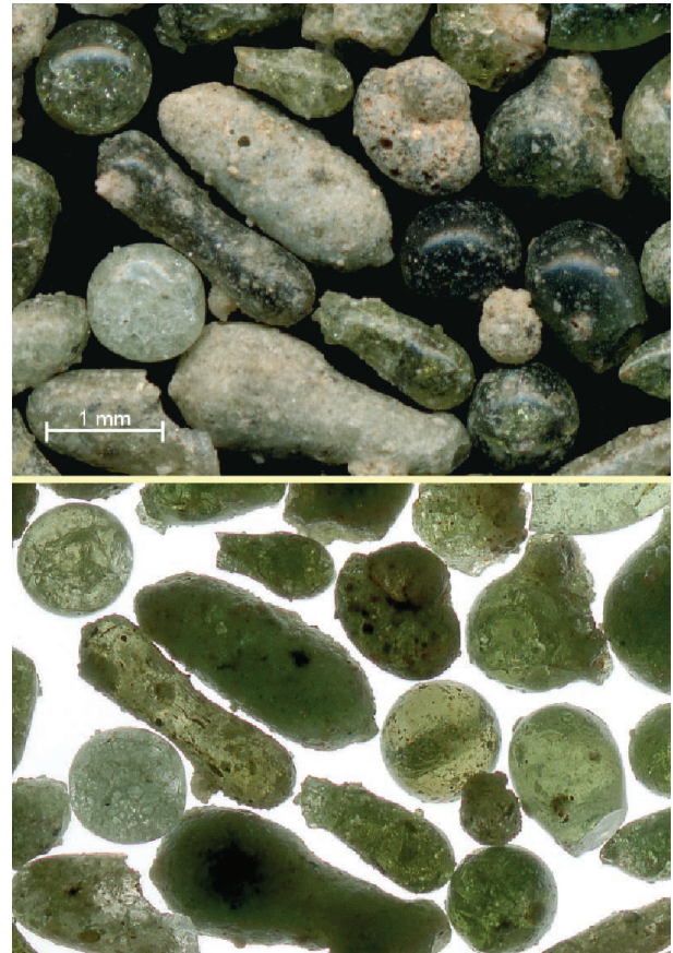
FIGURE 2. Trinitite beads and dumbbells. (top) Reflected light, (bottom) transmitted light. From Eby et al. (2010b), Figure 8.
